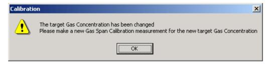
When the target Gas Concentration is set to zero, the user is warned by the following message:
