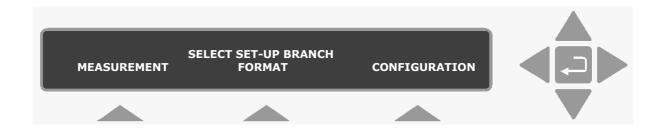
The display above is used through-out this manual. It assists you displaying the text on screen and by indicating which of the push-buttons can and should be pressed.
