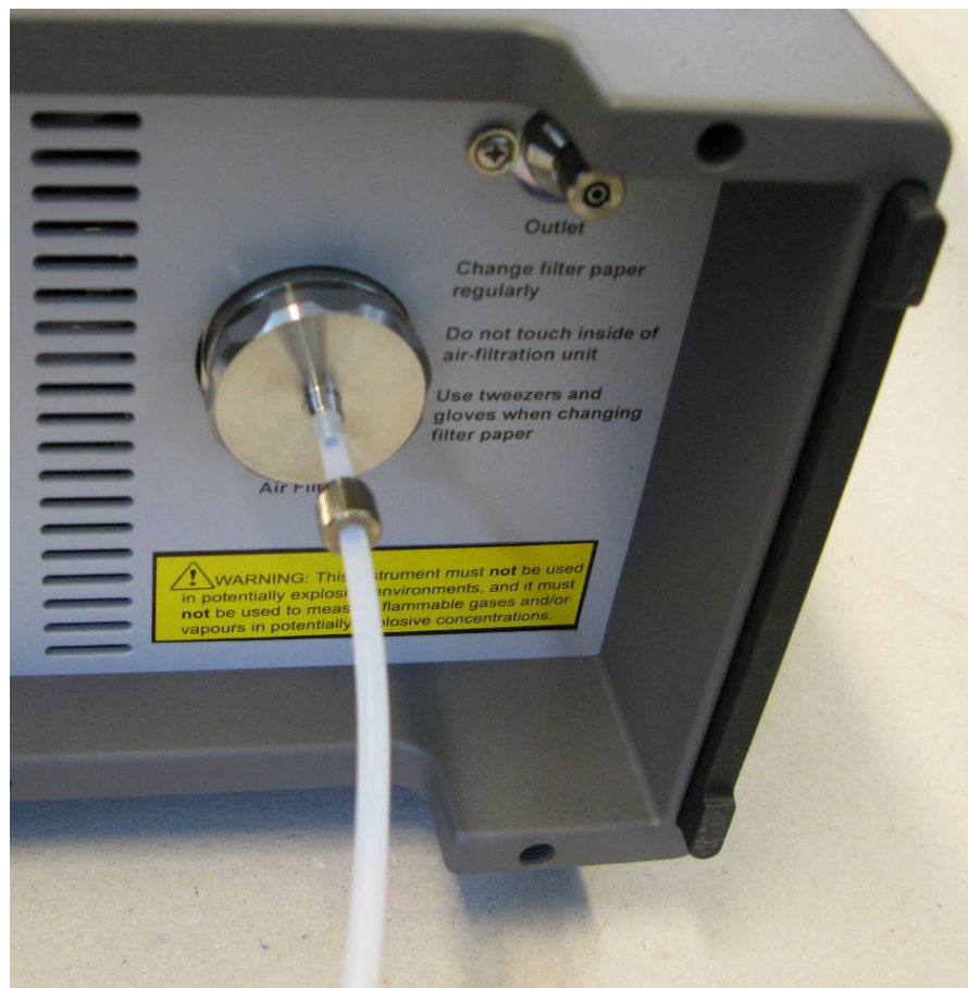
Fig.4.3 Attaching tubing to the air-inlet stub and the external filter
