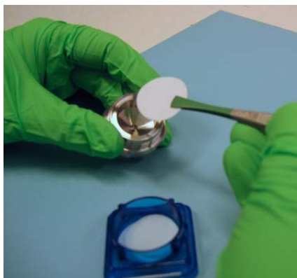
Fig.11.6 Placing a new filter-paper in the unit
