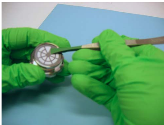
Fig.11.4 Removing the retaining disc and old filter-paper
