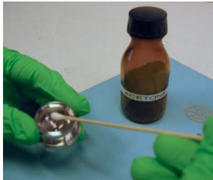
Fig. 13.5 Cleaning the surfaces of the internal air-filtration unit
