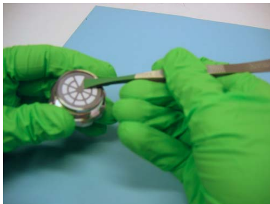
Fig.13.4 Removing the retaining disc and old filter-paper
