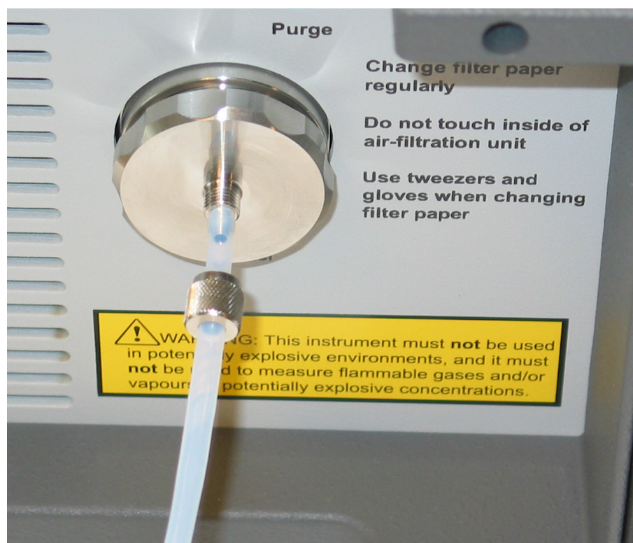
Fig.4.3 Attaching tubing to the air-inlet stub and the external filter
