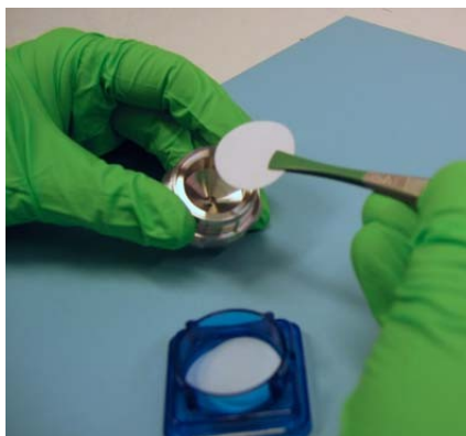
Fig. 13.6 Placing a new filter-paper in the unit
