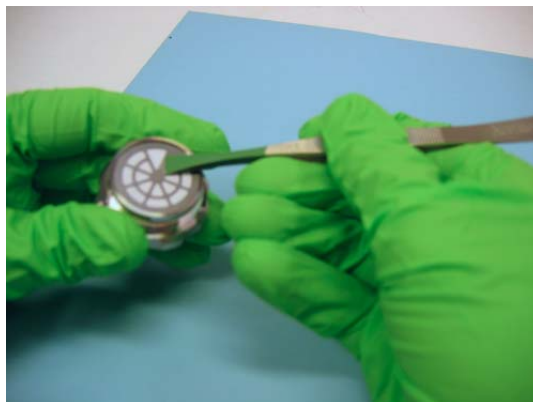
Fig.11.4 Removing the retaining disc and old filter-paper
