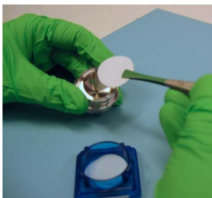
Fig.11.6 Placing a new filter-paper in the unit
