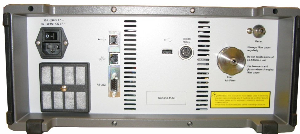
Fig.11.9 Back panel of the 1412i showing the ventilation unit
