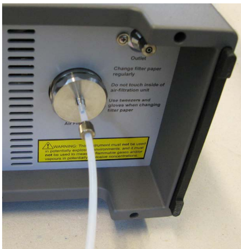
Fig.4.3 Attaching tubing to the air-inlet stub and the external filter
