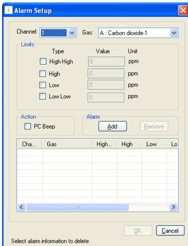
Figure 3.28 Alarm Setup for specific gases
