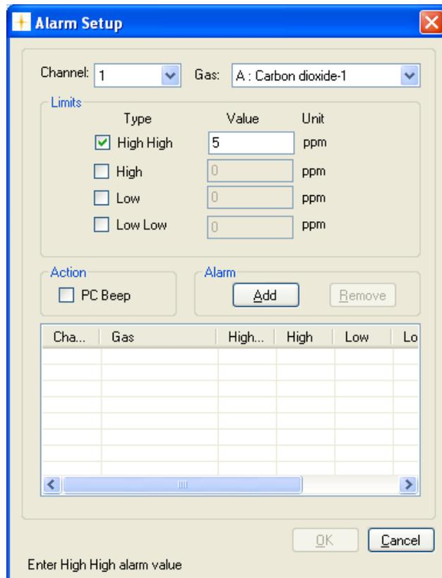
Figure 3.31 Select a type of alarm and type in a value for the gas concentration
