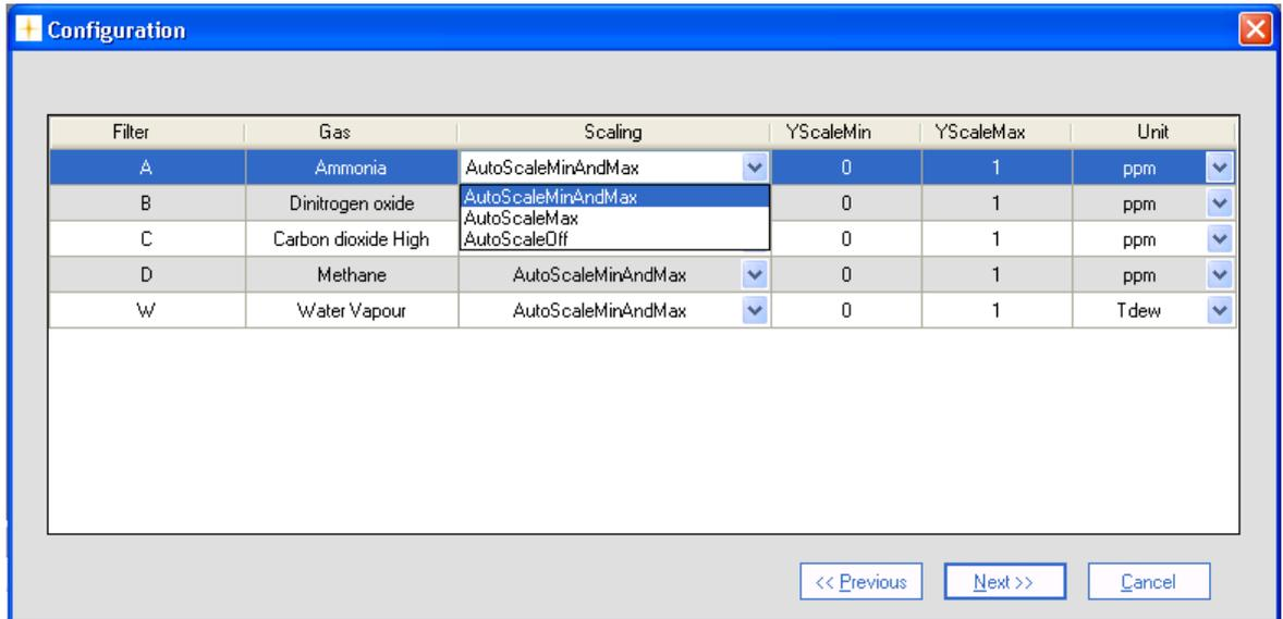
Figure 4.44 Setting the scaling of the axis
