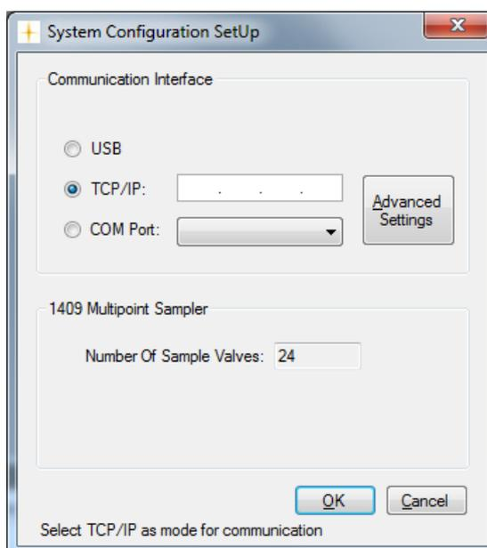
Figure 3.7 Select the TCP/IP communication interface.
