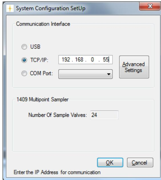
Figure 3.8 Enter the IP Address of the Gas Monitor.
