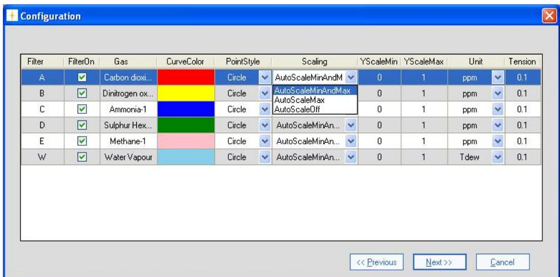
Figure 4.13 Setting the scaling of the axis
