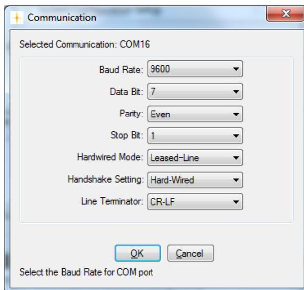
Figure 3.13 The RS-232 communication parameters
