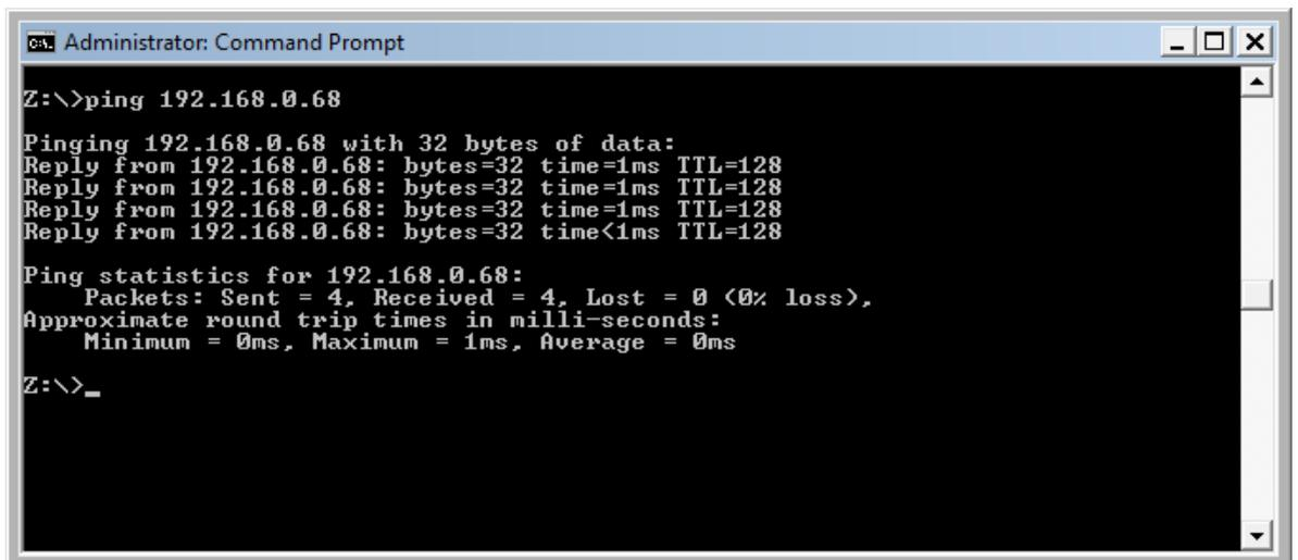
Figure 3.11 Ping reply from the Gas Monitor device.
