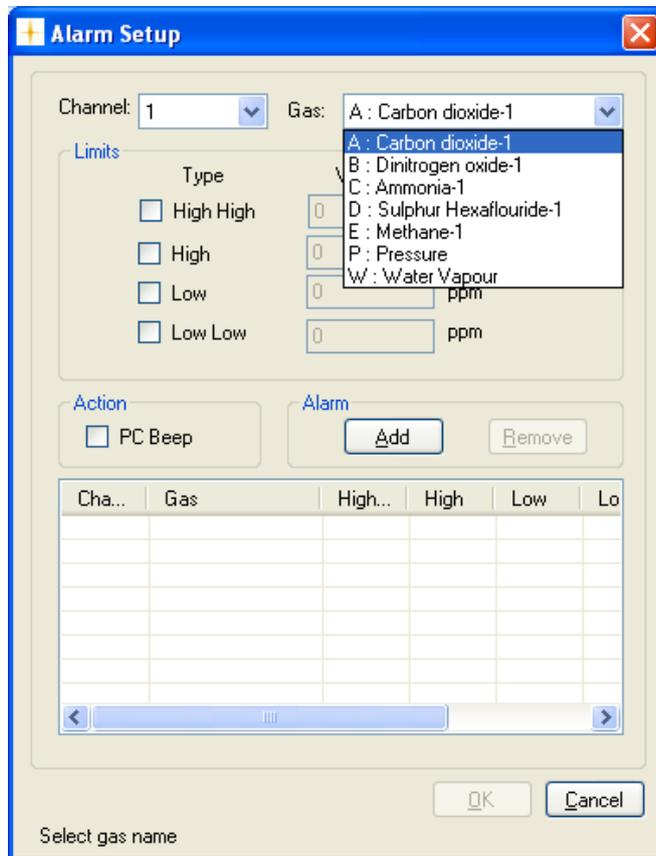
Figure 3.30 Select for which gas the alarm should be configured
