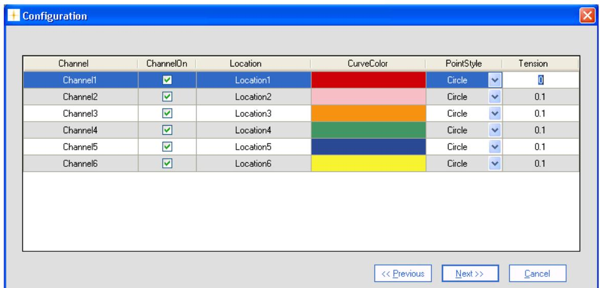
Figure 4.43 Define how hard/soft the lines between measurement points should be
