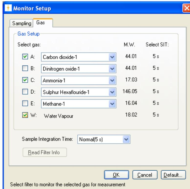
Figure 3.21 Monitor Setup, Gasses to be measured
