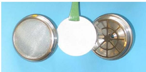
Moisten a cotton bud with pure acetone and use it to clean the surfaces of the unit, the retaining disc and the coarse air-filter. Refer to Fig.5.1.
