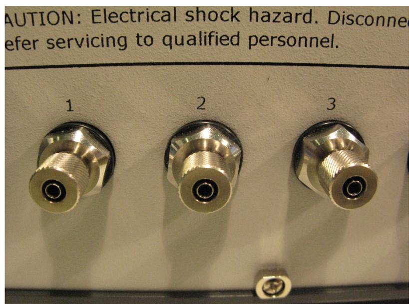
1. Remove the knurled nut from the mounting stub of the sampler channel you wish to use, on the front panel of the 1409.
