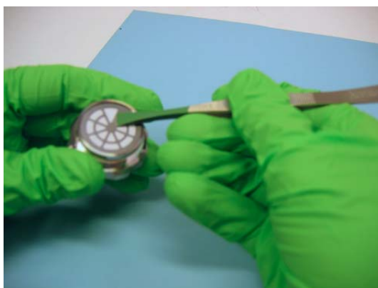
Fig.11.4 Removing the retaining disc and old filter-paper
