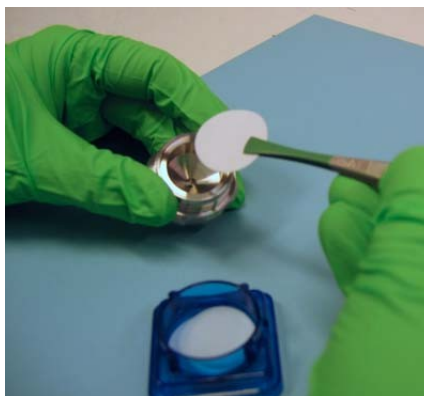
Fig.11.6 Placing a new filter-paper in the unit
