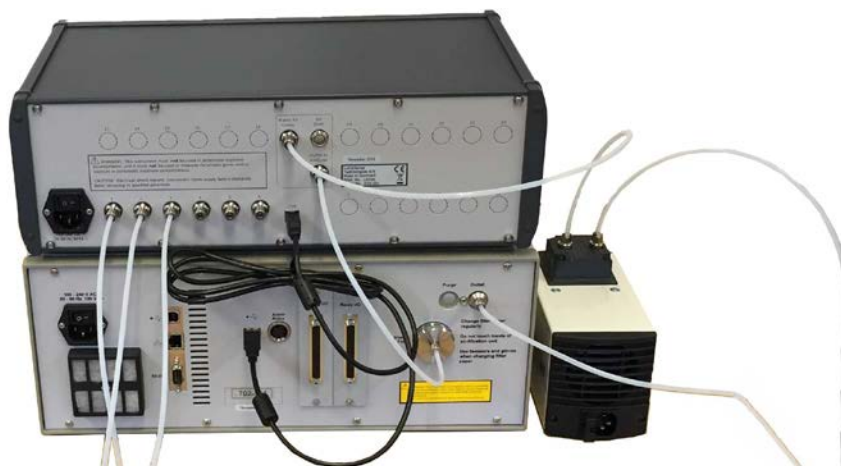
Figure 1. Tube and Cable connection with connection to an external pump.
