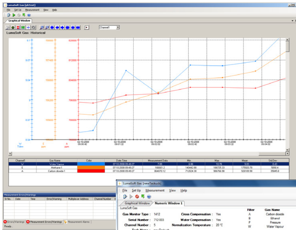
Figure 3: In the channel view mode, the graphical window shows up to seven graphs. The user selects the data plotted, the scaling, the style and the color of the lines and the background to build the graphical window.
