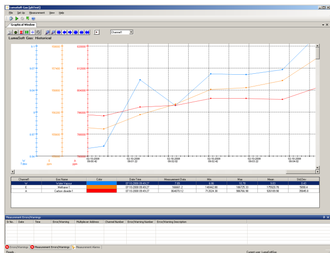
Fig. 1 The graphical window shows up to seven graphs. The user selects the data plotted, the scaling, the style and the color of the lines and the background to build the graphical window
