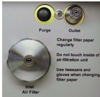
Fig.13.1 The internal air-filtration unit mounted on the back panel of the monitor.
