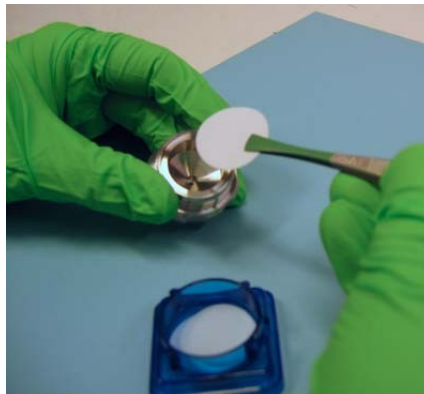
Fig.13.6 Placing a new filter-paper in the unit
