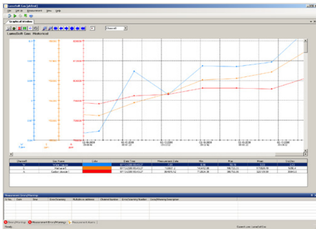
Fig. 1 The graphical window shows up to seven graphs. The user selects the data plotted, the scaling, and the style and color of the lines and background to build the graphical window.
