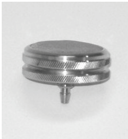
Fig.11.3 The external air-filtration unit UD5023 used with the Monitor, (optional accessory)
