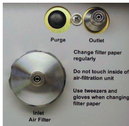
Fig.11.1 The internal air-filtration unit mounted on the back panel of the monitor.
