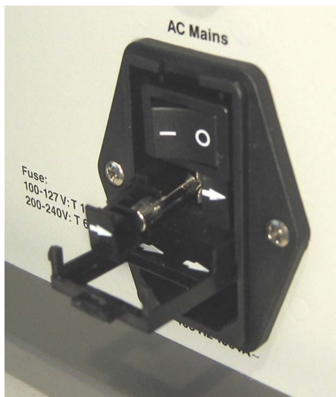
Fig.2.2. Inserting the fuses into the 1303's fuse holder
