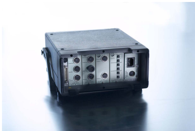
Fig. 1.2 Back – 1221 Thermal Comfort Data Logger
