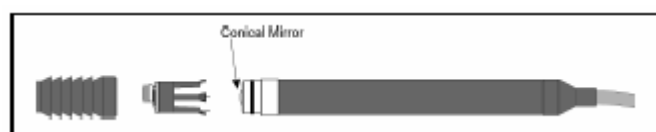
Fig 3.7 Disassembling the MM 0037 Transducer
